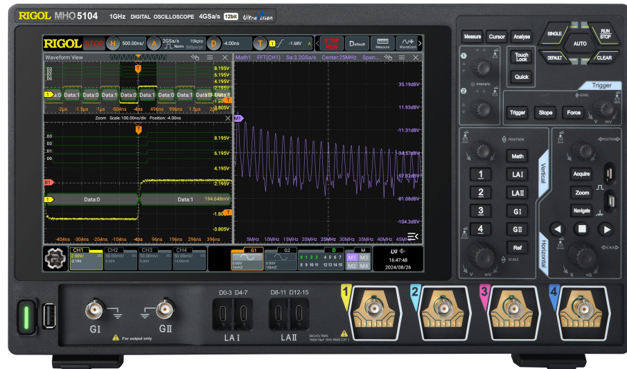
Figure 4.2 MHO5104 Front Panel
